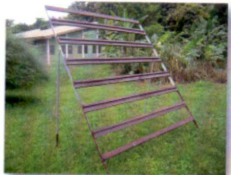
Plate 4: Wood and metal mix rake for exposure tests
