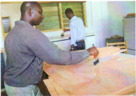
Plate 14: Brushing of plywood with adhesive
