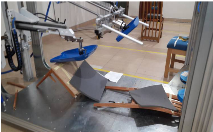
Plate 41: A chair failed at test
