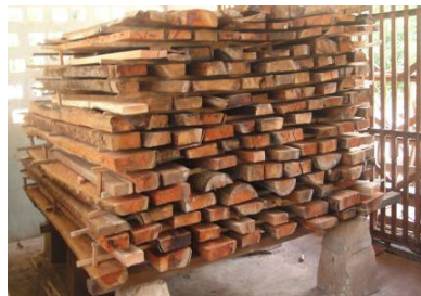
Plate 12: Eucalyptus alba/robusta lumber stacked for air drying
