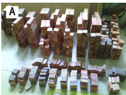
Plate 15A & B: Prepared specimens from Eucalyptus species for mechanical strength tests
