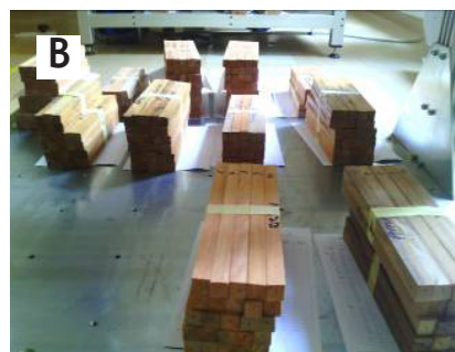
Plate 15A & B: Prepared specimens from Eucalyptus species for mechanical strength tests
