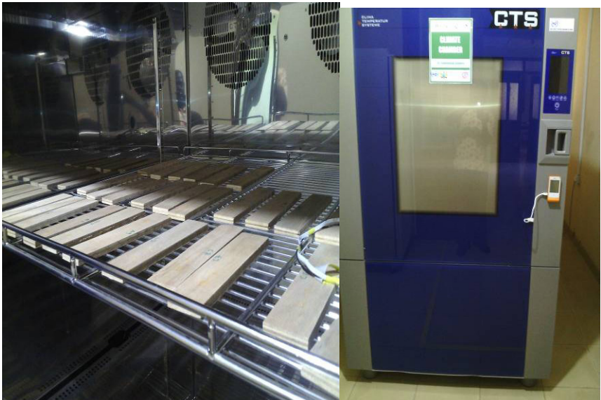
Plate 44: Specimens for round robin test being conditioned in a climate chamber
