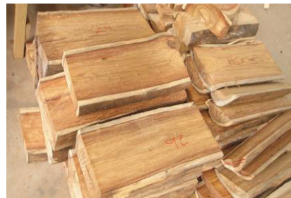
Plate 14: Eucalyptus samples being prepared for physical tests
