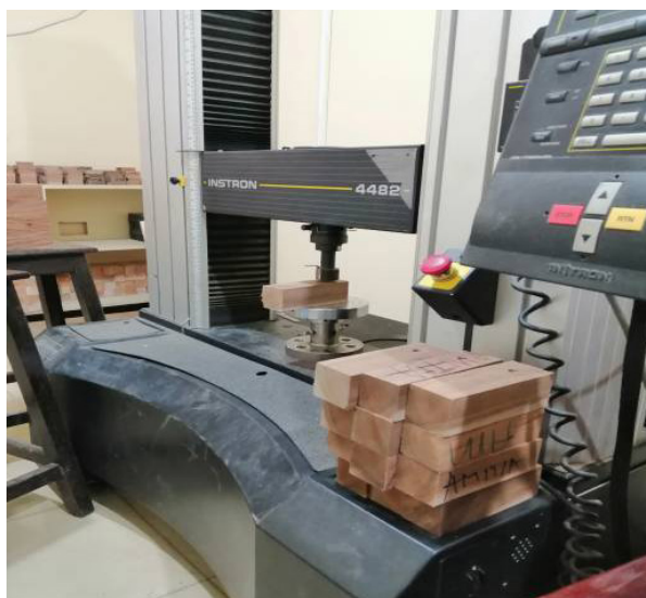
Plate 16: Mechanical strength testing of prepared specimens from Eucalyptus species
