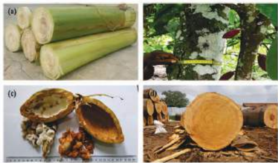
Plate 37A-D: Materials collected for production and characterization of particulate panels. Musa paradisiaca pseudostem (a); Theobroma cacao stems (b); Theobroma cacao pods (c); Ceiba pentandra wood (d).
