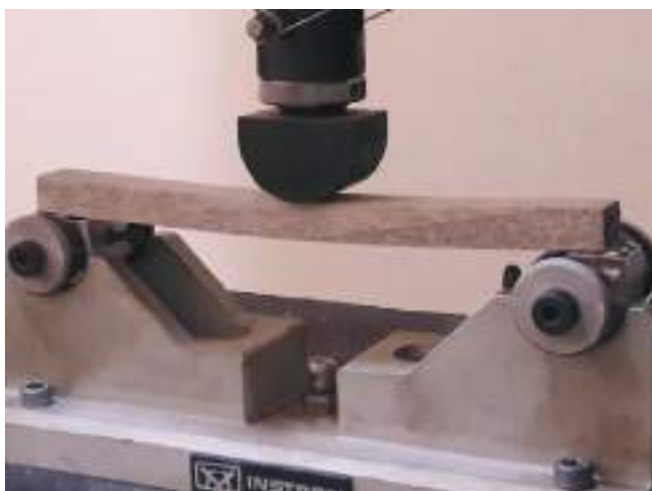
Plate 36: Static bending test on a wood specimen
