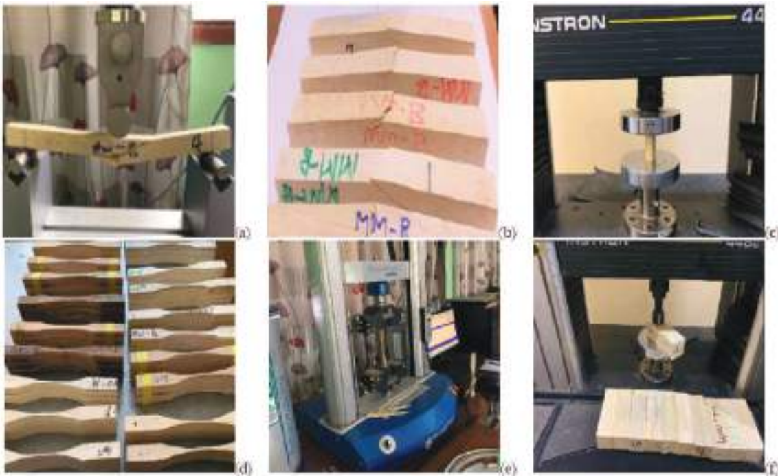
Plate 39A-F: Mechanical properties assay: static bending (a) and specimens after test (b); determination of compressive strength parallel to the grain (c); specimen used for tensile strength parallel to the grain tests according to standard (d) and tensile strength test (e); Janka indentation tests (f).
